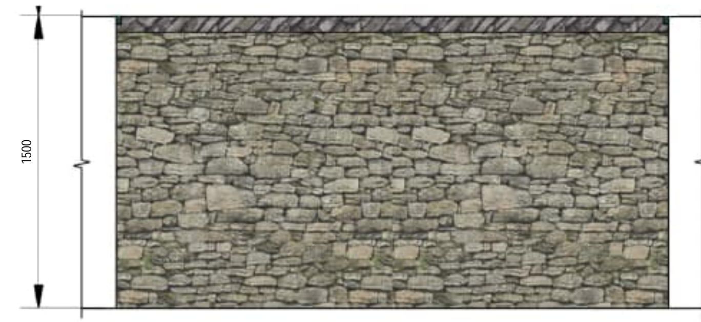
PROPOSED DRYSTONE WALL DETAIL
